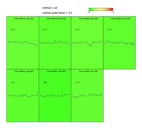
In this plot the fingerprints for each of the 7 tubes is shown in a grid. The color of the grid square for a tube indicates the standard deviation of the normalized and log-transformed fingerprint feature vector for that tube according to the color scale at the top of the figure. The standard deviation value is printed in the grid square.
