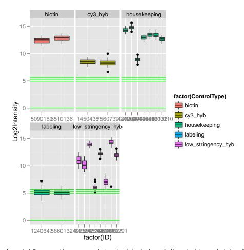
In quickSummary the mean and standard deviation of all control types is taken for a specified array, using intensities of all beads that correspond to the control type. Note that these summaries may not correspond to similar quantities reported in Illumina's BeadStudio software, as the BeadStudio summaries are produced after removing outliers (see later).
