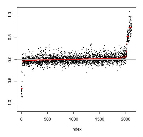
Change-points are often found due to local trends in the data. An undo method is needed to get rid of unnecessary change-points. Below all splits that are not at least three SDs apart are removed. The following plot shows that all splits not corresponding to the gold standard results have been removed.
